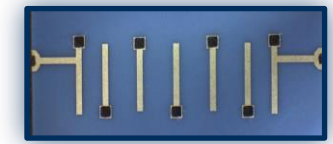
Above: 9.5 GHz Bandpass filter response. Size: 9 x 7 mm.
